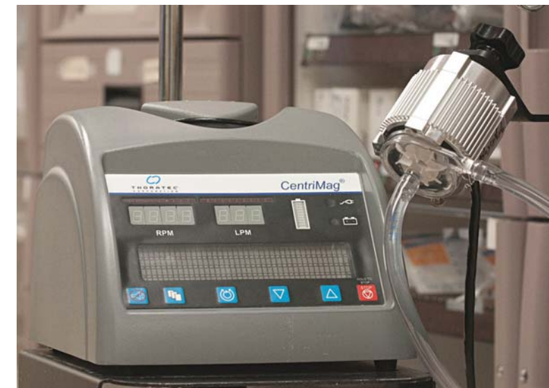
The external VAD used at Baystate Medical Center—the CentriMag by Thoratec Corporation—is an external device, about six inches in diameter, that sits next to the patient’s bed.
